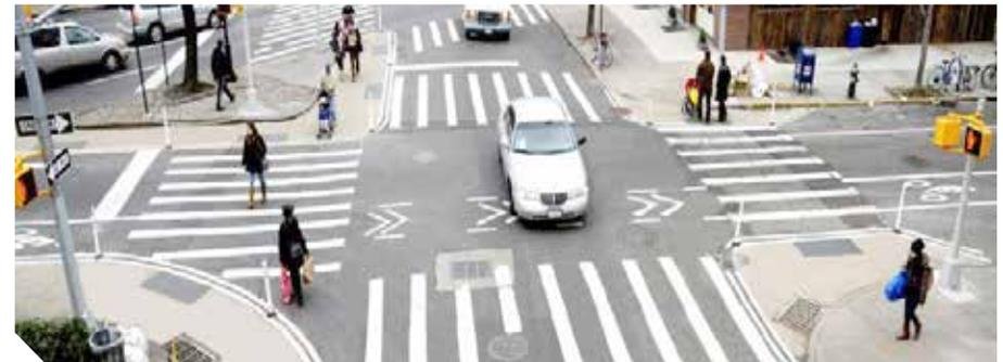
In this picture you can see how the original curb has been extended and re-shaped. A tighter turning radius makes drivers take the turn slowly and creates a shorter crossing distance.
